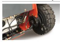
The lifting and Driving with the AC motor, Front axle with wet brake, free maintenance
