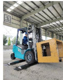
The truck passed simulation experiment of bumpy road.
