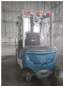
IPK4 waterproof: the vehicle is powered on to simulate a 15min short-time 5000L rainstorm test, and the vehicle can continue to run without failures.
