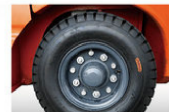
Tyre with plying rating 14
