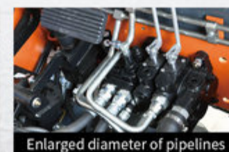
Enlarged diameter of pipelines
