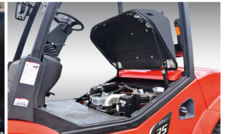
Engine cover with large opening angle, large maintenance space
